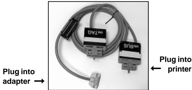
Figure 3-2. CHANNEL-OUT cable
